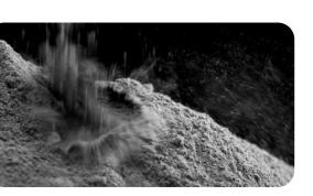
CaD is a powerful agent for hot metal desulfurization based on finely ground Calcium Carbide (CaC<sub>2</sub>) powder.
