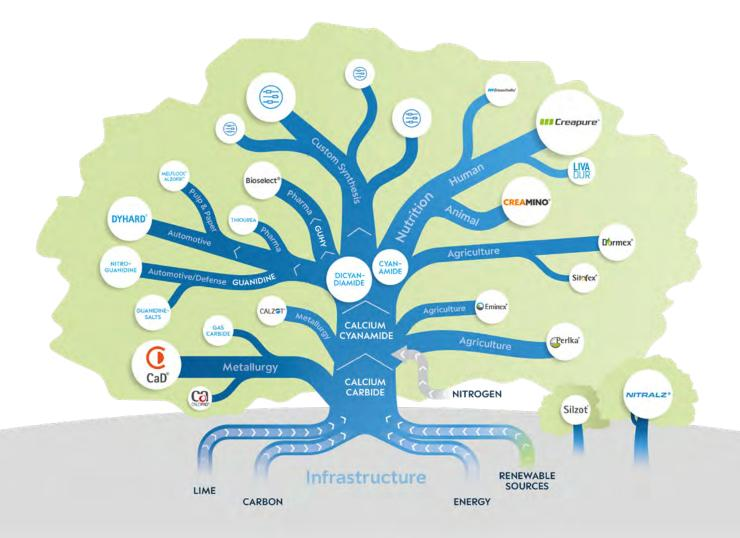
The main products of the Alzchem Group are based on the same raw materials, namely lime and coal. Along the calcium carbide/calcium cyanamide (NCN) chain, Alzchem integrates many processing and refining steps to create the respective products in the Basics & Intermediates and Specialty Chemicals segments.
